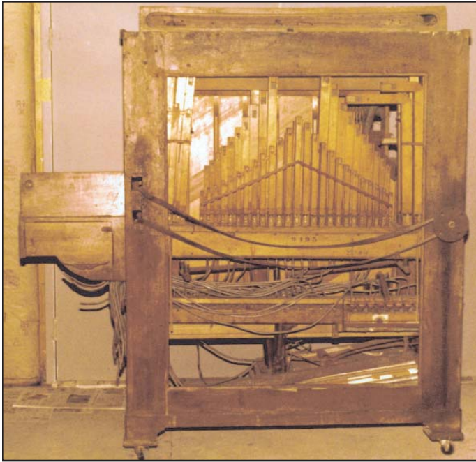
Figure 16. This view of the back shows the unusual drive configuration and the back-facing pipework of the Piano-Quartet .
